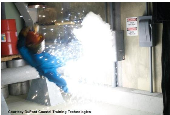
Non-arc resistant equipment designs do not control direction of thermal energy
