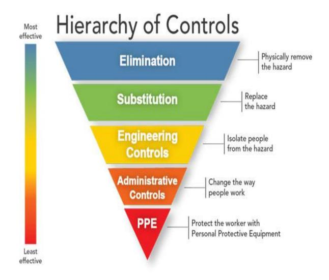
The idea behind this hierarchy is that the control methods at the top of graphic are potentially more effective and protective than those at the bottom. Following this hierarchy normally leads to the implementation of inherently safer systems, where the risk of illness or injury has been substantially reduced.
