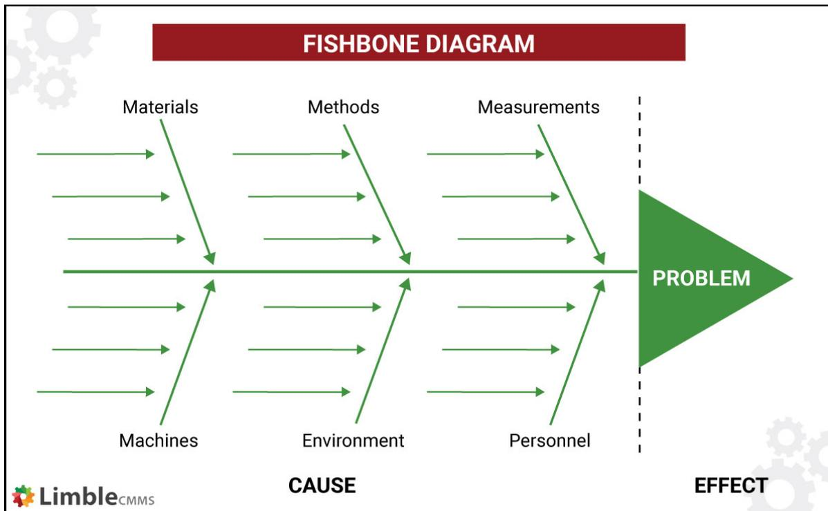
The 5 M framework—aka. a fishbone diagram—from the [Toyota Production System](#) is utilized for RCA with the Ishikawa method.
