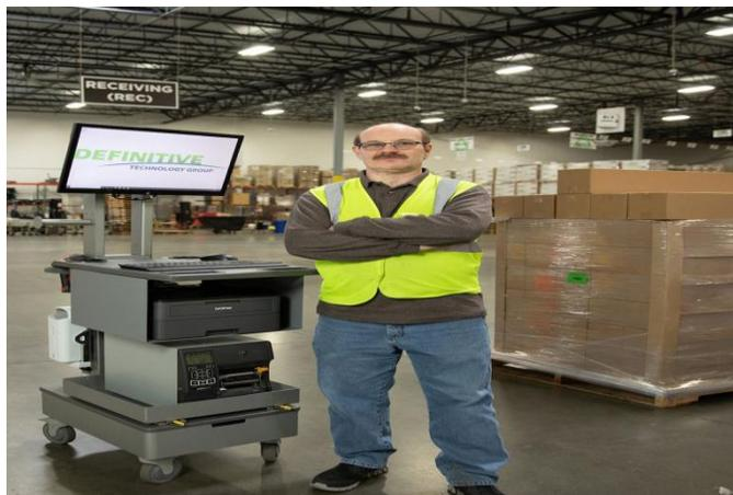
Mobilized power workstations help to reduce motion waste, and enable more efficient picking, packing, and receiving in the warehouse.
