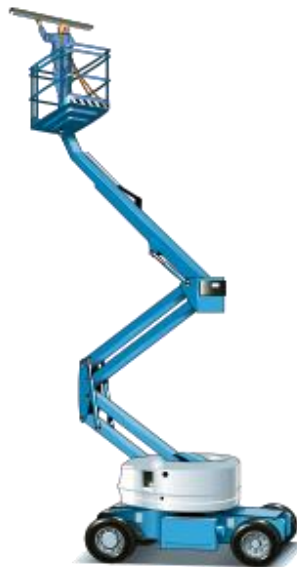
A mobile elevating work platform
