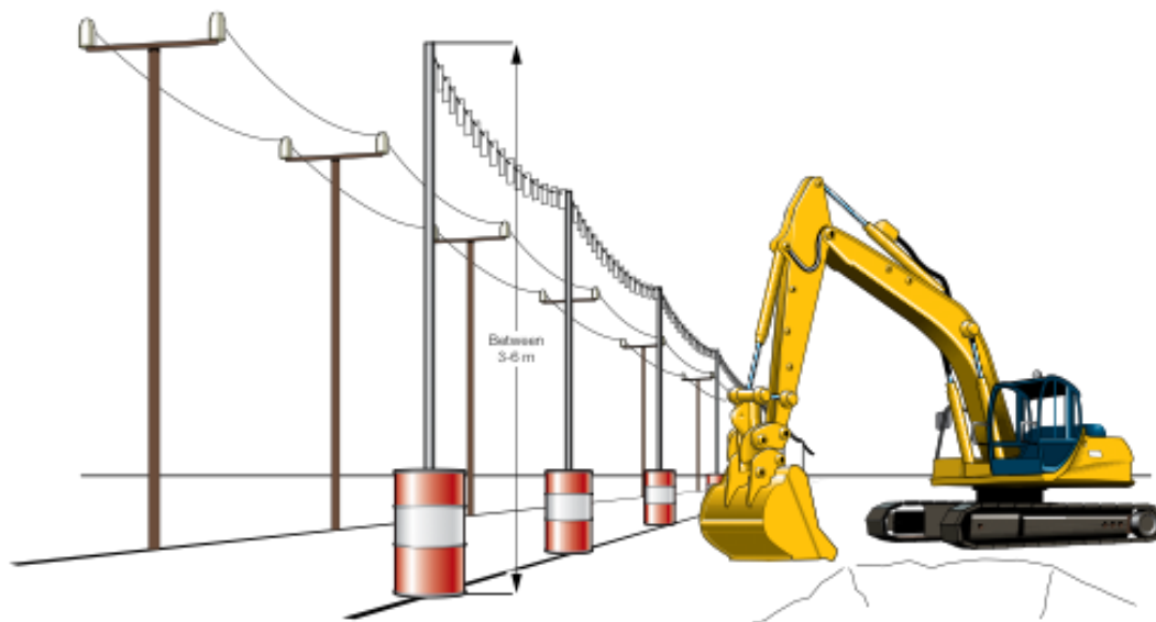
Figure: Ground-level barrier for plant working near an overhead power line
